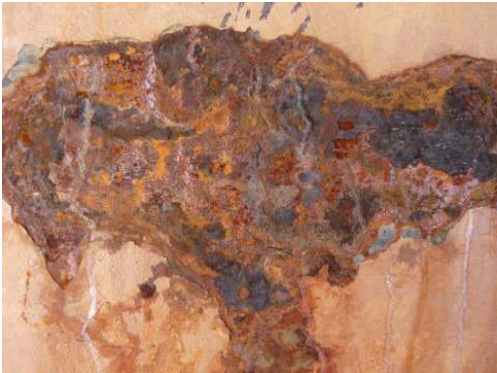
Corrosion under insulation (CUI) – Close up
