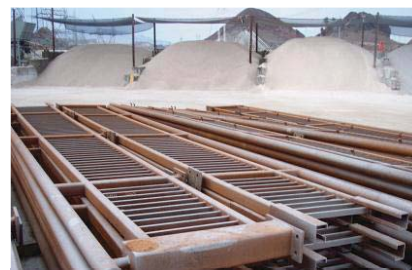
Steel railings were allowed to develop flash rust in preparation for the Rust Grip® application.
