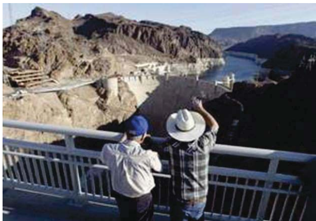
The observation deck expects 3-5 million visitors each year. Super Therm® will protect them from possible burns from the railing's hot steel surface, which can reach over 150°F.
