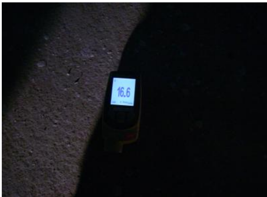
Surface profile before removing the scale rust. Up to 16.6 mils or 420 micron.
