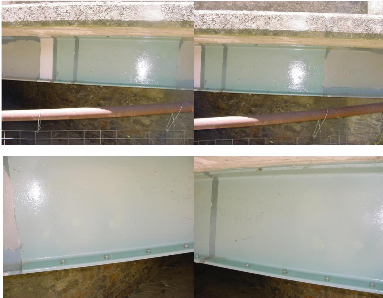
**Round spots mark the area where pull dollies were attached to perform pull tests.**
